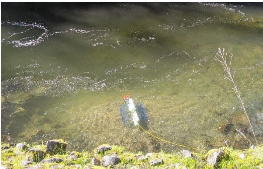
Horizontal deployment of a hydrophone in Hood River
